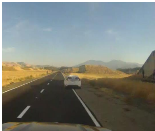
Figure 14: Lateral placement of DRI Soft Car 360® Image Source: AAA
