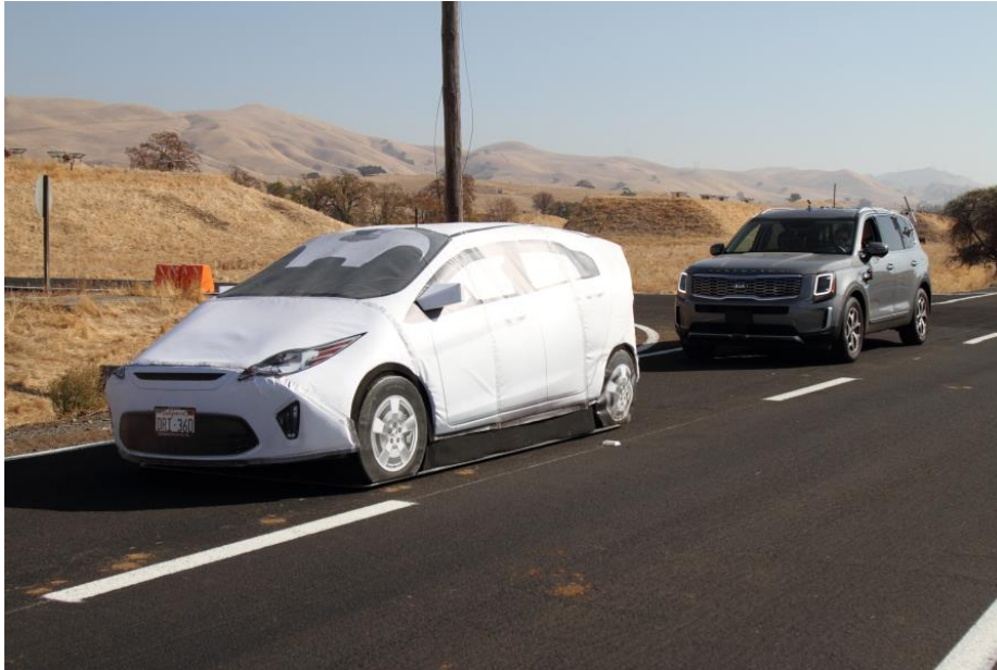
Figure 8: DRI Low Profile Robotic Vehicle Image Source: AAA
