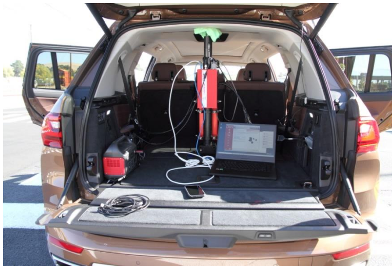
Figure 2: Test vehicle outfitted with closed-course instrumentation Image Source: AAA
