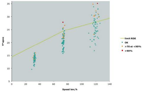
Figure 3 : Dynamic drives for large vehicles on RDE limit curves
