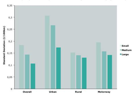
Figure 10: Standard deviation across Protocol results, for all valid trips, by vehicle size
