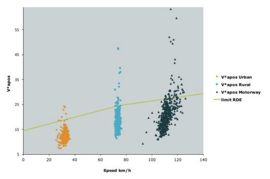
Figure 2 : 340 tests on the high dynamic condition limit curve
