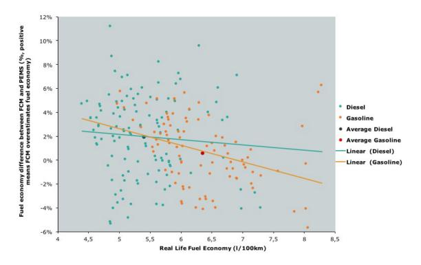
Figure 15: Comparison between Fuel Consumption Meter and PEMS measurements
