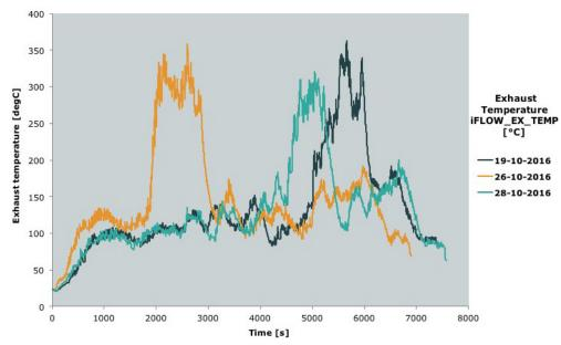
Figure 28 : Example of regenerations detected during various tests
