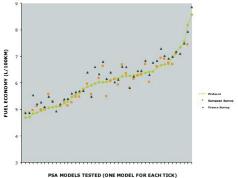
Figure 5: Protocol results compared with internal PSA surveys
