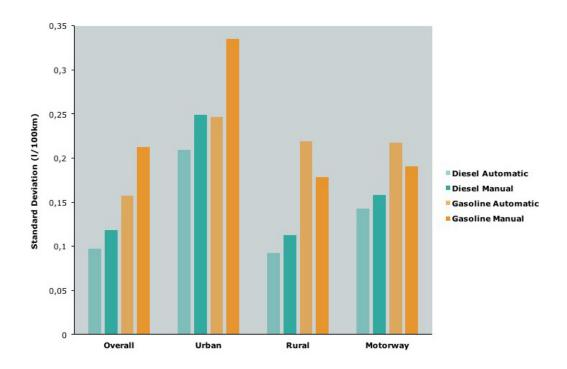
Figure 9: Standard deviation across Protocol results for all valid trips, by fuel and transmission type
