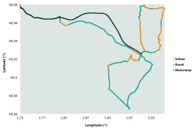
Figure 1: Urban, rural and motorway sections of the Protocol route in the outskirt of Paris
