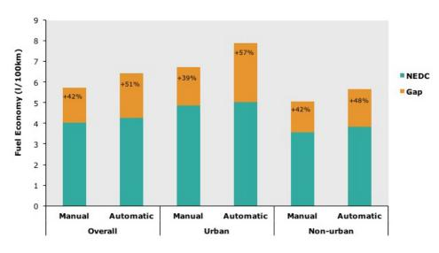
Figure 22: Protocol gap by transmission type
