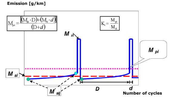
Figure 29 : Ki Factors calculation procedure as per UNECE regulation 83<sup>20</sup>.
