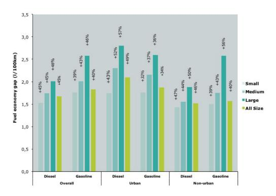
*Figure 16: Fuel economy gap between the Protocol and certification, by fuel type and vehicle size.*
