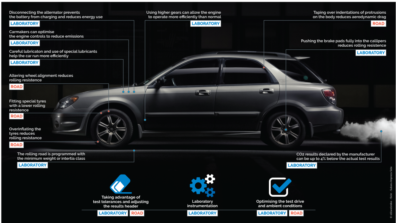
Fig 4: Common ways carmakers manipulate tests for CO 2 emissions and fuel economy
